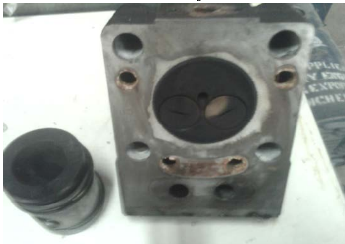
Figure 2: Zirconium Oxide coated piston and head
