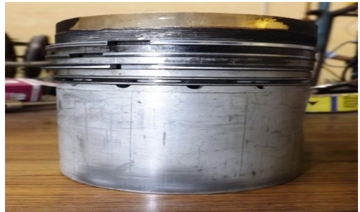
Figure 3: Photographic view of Normal Aluminum piston
